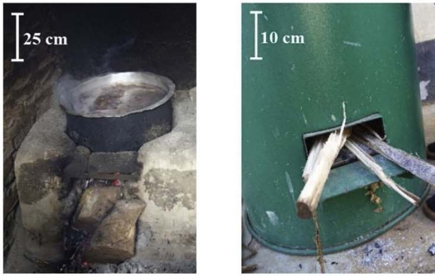
Fig. 3. Biomass fuel size differences between the semi-improved boiling method (left) and the InStove Water Purifier (right).
